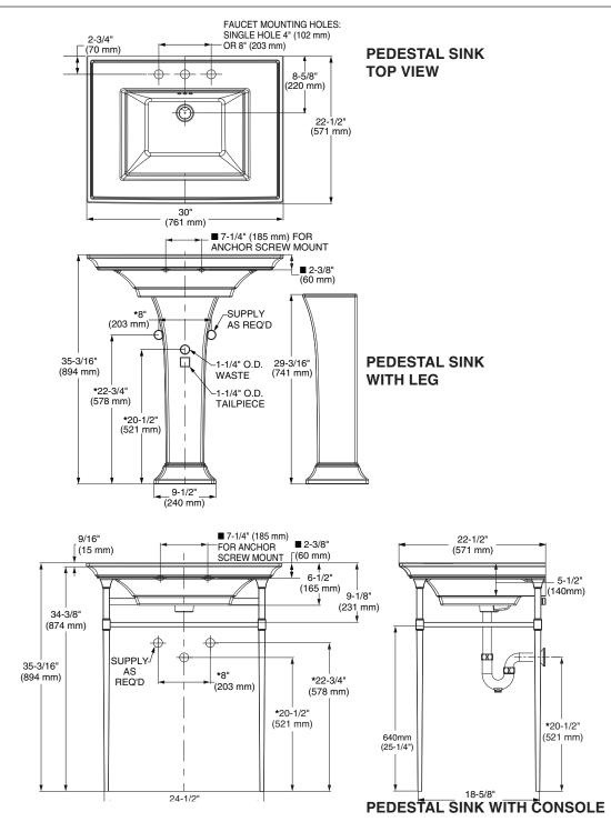
NOTES: \* DIMENSIONS SHOWN FOR LOCATION OF SUPPLIES AND "P" TRAPS ARE SUGGESTED. ■ SUITABLE FOR REINFORCEMENT ONLY. ACTUAL DIMENSIONS MUST BE TAKEN FROM FIXTURE. FITTING NOT INCLUDED AND MUST BE ORDERED SEPARATELY. PROVIDE SUITABLE REINFORCEMENT FOR ALL WALL SUPPORTS.
